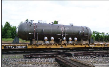
Pressure Vessels (Steam Drum)
