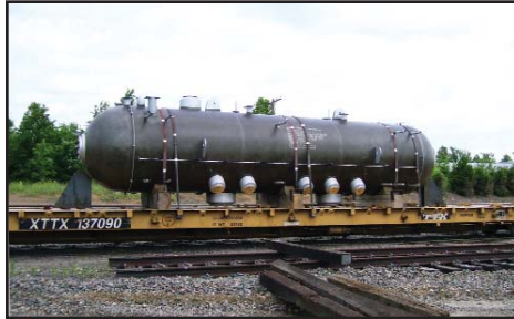
Pressure Vessels (Steam Drum)
