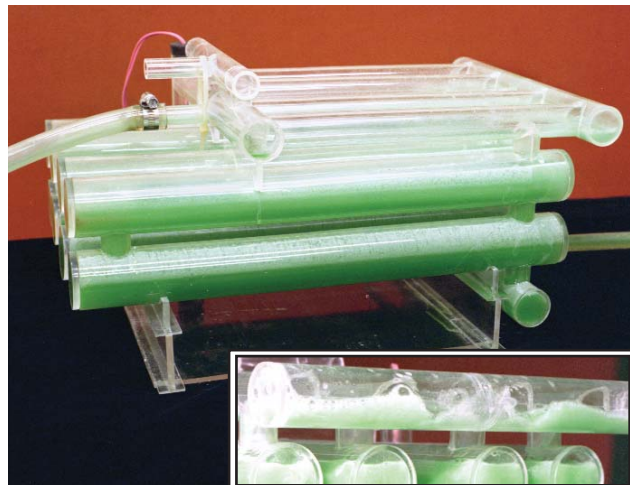
Detail of distribution header
