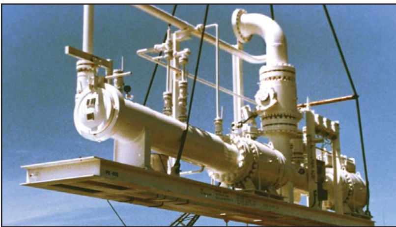
Trap with Patented Closure (Skid Mounted for Export)
