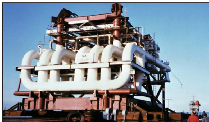
Slug Catcher (Offshore Facility Utilizing Headers)
